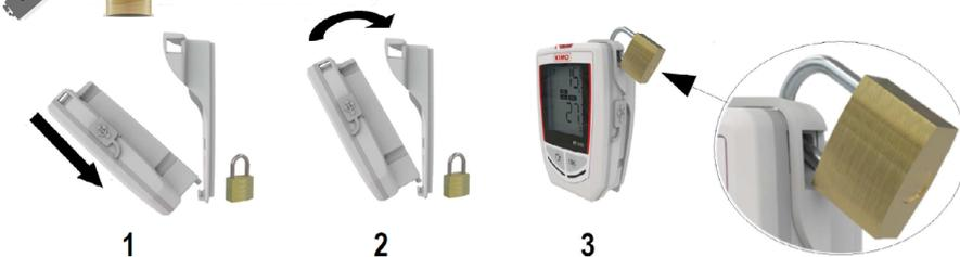
Mount the safety lock support on the required place.
